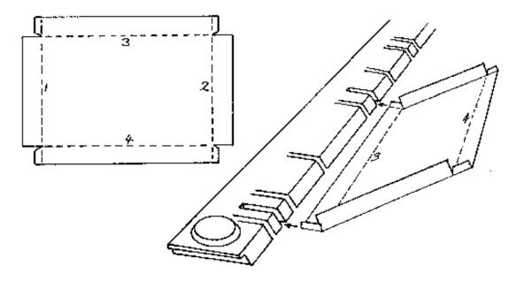
The advantages of the slotted clampbar over the set of short clampbars for making trays are that the bending edge is automatically aligned to the rest of the machine, and the clampbar automatically lifts to facilitate the insertion or removal of the workpiece. (Never-the-less, the short clampbars can be used to form trays of unlimited depth, and of course, are better for making complex shapes.)
